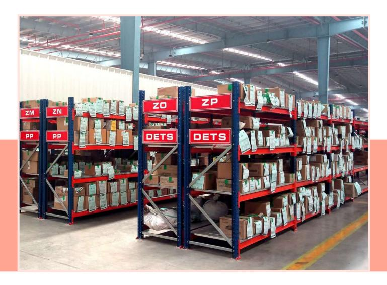
Designed for warehouses where goods are manually placed and removed from shelves, our system is modular—that is, shelves may be simply rearranged and expanded depending on the products to be stored. Shelf height can be adjusted to a pitch of 50mm. These Shelving solutions also make the best use of warehouse height by making higher levels mechanically accessible.
