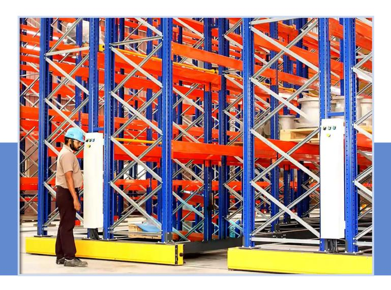
Craftsman Mobile Pallet Racking System is equipped with emergency stop and manual release buttons and a modern control system that controls, electric drive units for mobility, and various sensors for access and safety to ensure trouble-free operations, thus creating a safe operational environment in your warehouse. The system can be operated by the push buttons on the racks and/or with remotes. Mobile pallet racking systems are ideal for cold storage applications.
