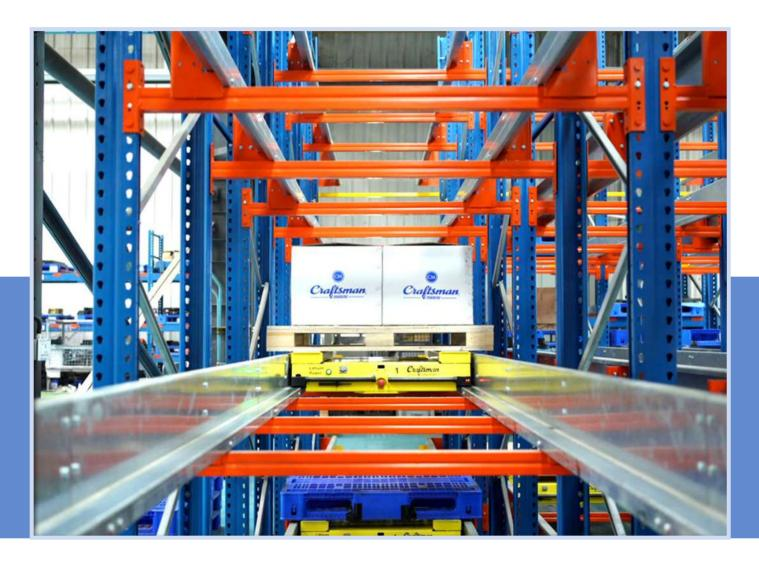
Our Radio shuttle racking system is compatible with all major types of forklifts, including counterbalance, narrow-aisle, and swing reach lifts. Furthermore, the safety of the racking structure is ensured as lift trucks never actually enter the racking system like Drive-In.
